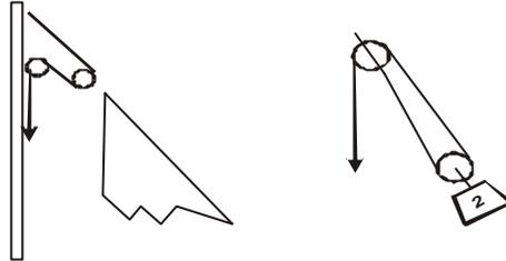
A peak halyard with blocks all over the place, but again consolidating the elements on the fixed and moving parts resolves the tackle into a double purchase with 4:1 advantage
