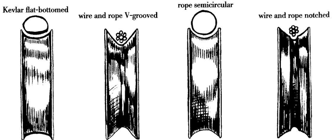
score, which needs to be different for traditional rope, wire rope, and modern composite ropes. The picture - from the rigging manual - shows the differences. Please note that if you have a notched wire & rope sheave, and then convert to an all rope halyard, it will chafe like mad on the edges of the notch.
