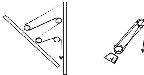
Finally a double-ended main-sheet. Assuming one end is cleated, then hauling on the other will give you 4:1 advantage. The sheave nearest the cleated end does nothing at all, and so doesn't feature in the addition.
