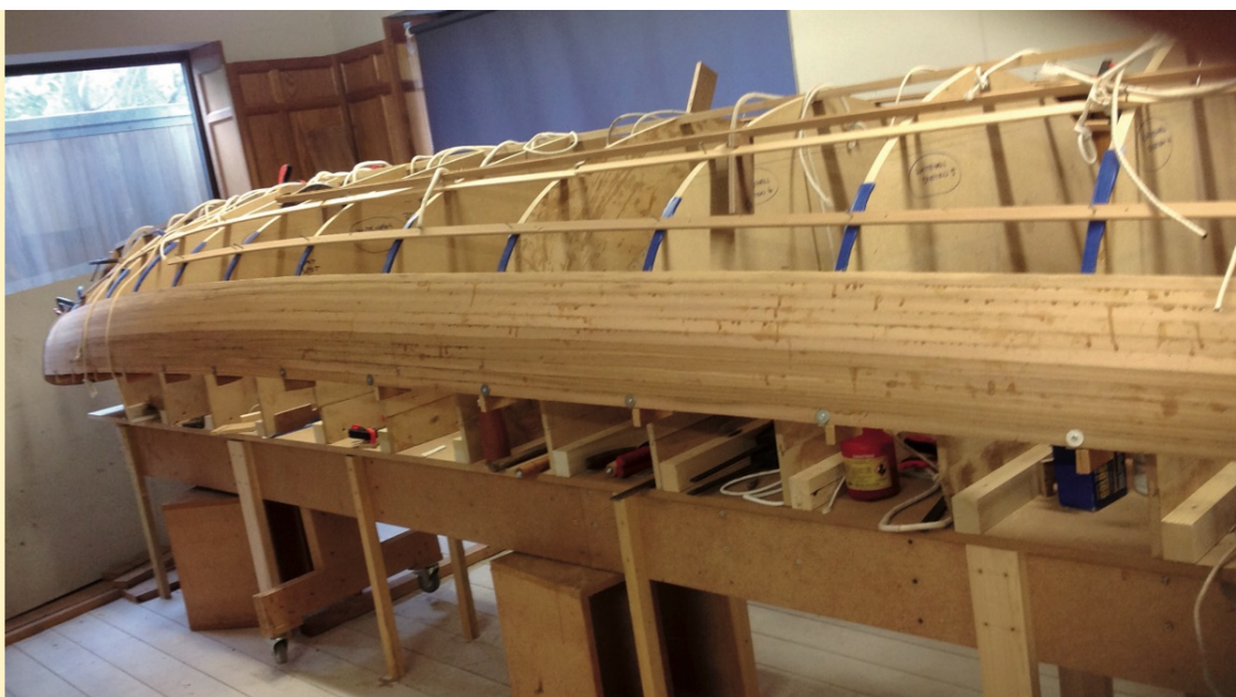
Modern wood construction: building a lightweight rowing skiff using cedar strip planks edge-glued together, often using epoxy... but not always. Photographs: www.cedar-strip.co.uk
