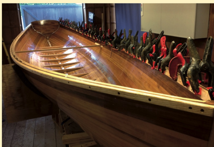
Modern wood construction: building a lightweight rowing skiff using cedar strip planks edge-glued together, often using epoxy... but not always. Photographs: www.cedar-strip.co.uk
