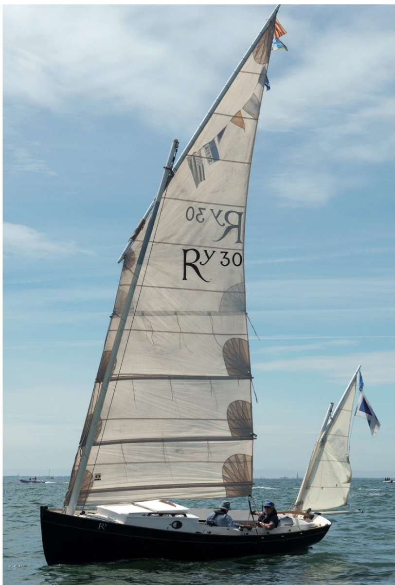
Carbon spars on Romilly, a modern lugger designed by Nigel Irens. Photo: Kathy Mansfield
