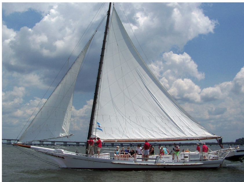
Working craft of the Chesapeake Bay like Nathan of Dorchester, a skipjack typically used for oyster dredging, used heavily raked masts to avoid the need for running backstays. Photograph: Dorchester Skipjack Committee Inc.
