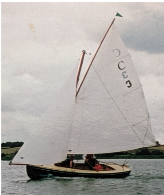
Right: Orwell OD reverted to gaff rig – which proved 10% faster
