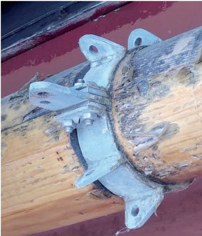
Left: Another sorry-looking stick but the substantial shoulder has made sure the galvanised mastband has not slipped. Right: A smarter mast with a through-bolted stainless steel mastband but there are signs of slippage and rotation.
