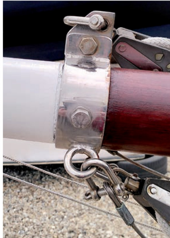
Left: Another sorry-looking stick but the substantial shoulder has made sure the galvanised mastband has not slipped. Right: A smarter mast with a through-bolted stainless steel mastband but there are signs of slippage and rotation.
