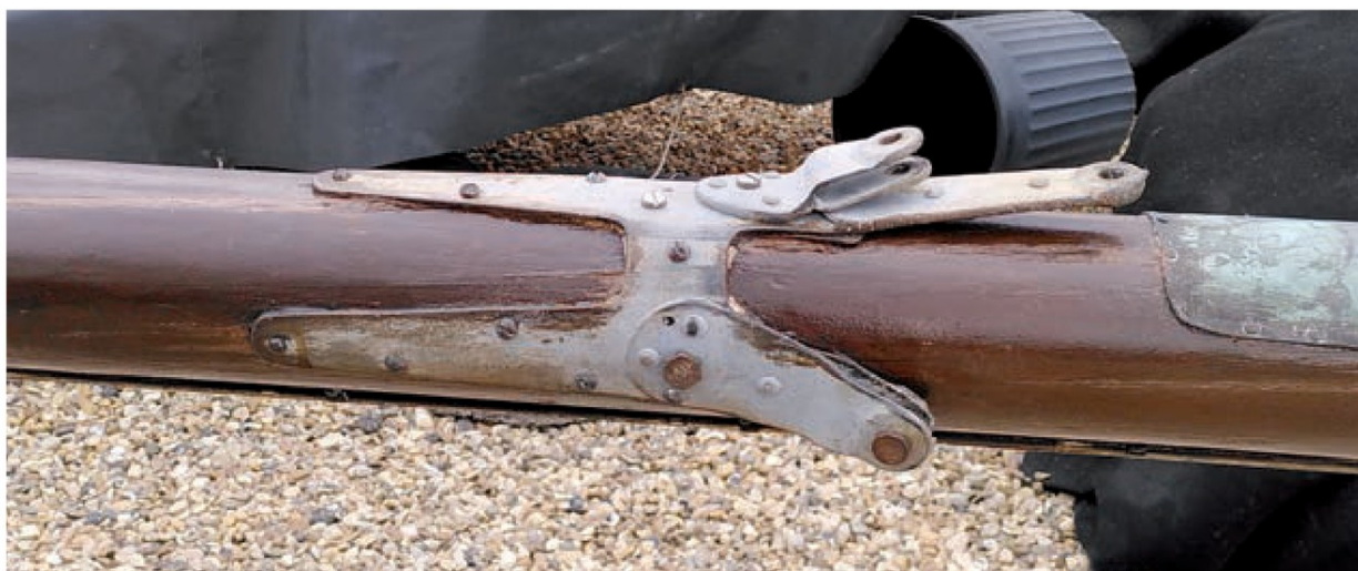
If a mastband cannot be fitted – because the mast has a sailtrack or for other reasons – then large area plates with plenty of screws and a though-bolt or two seem to be what's required
