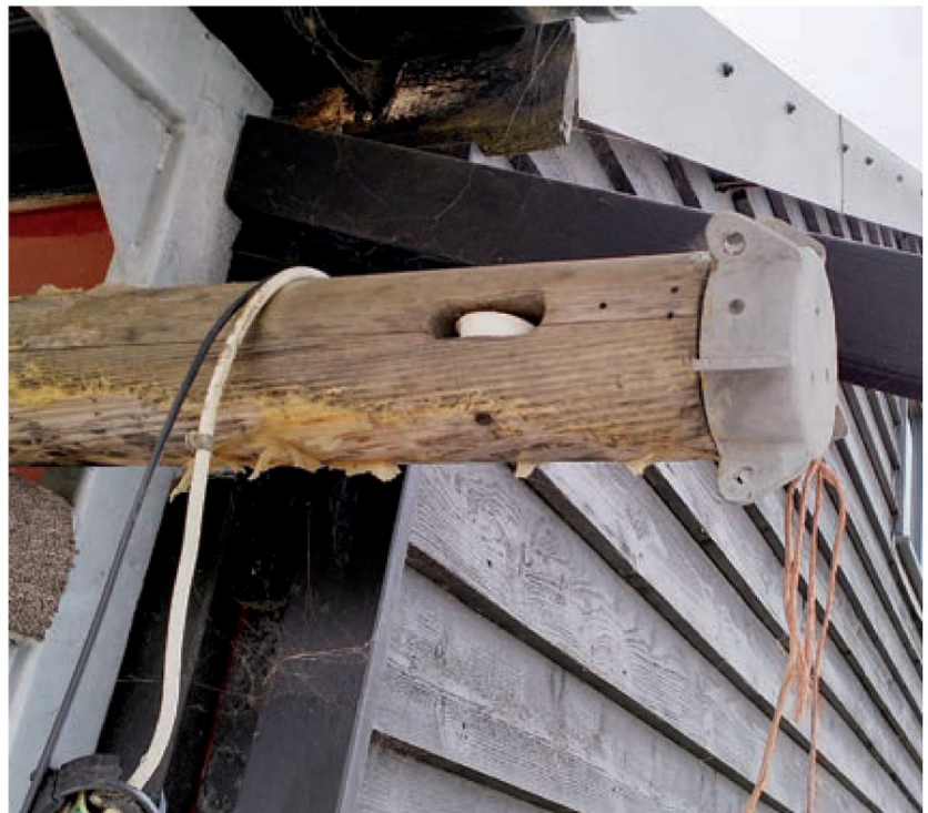
Above: Our sample modern gaffer: the late Ed Burnett's 30' (9.1m) Zinnia Below: This old wooden mast has clearly seen better days but the mastband is capped and it sits on a shoulder; both ensure it stays at the top of the mast.
