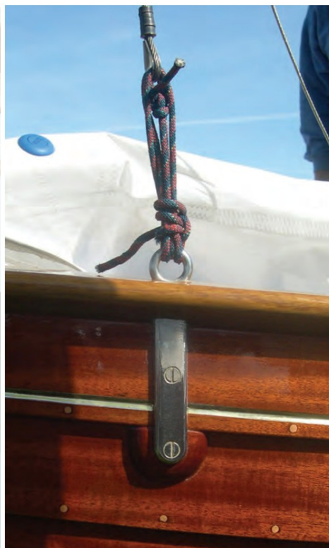
Left: Channels spread the load on an 1880s Nicholson design. Right: Chainplate on a clinker International 12 dinghy.
