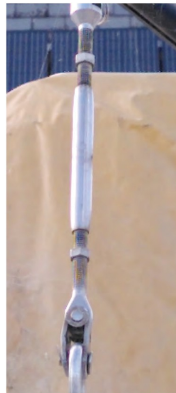
A rigging screw horror show L to R: At the end of the tether; Rusty threads, top one seized; Locknuts are for wimps.
