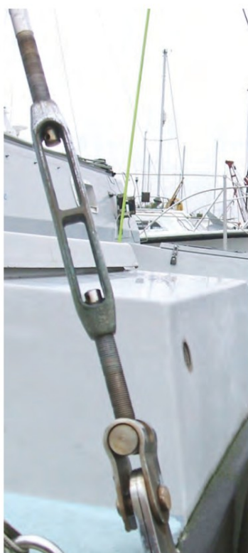
A rigging screw horror show L to R: At the end of the tether; Rusty threads, top one seized; Locknuts are for wimps.
