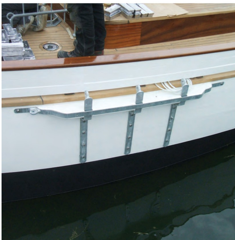
Left: Channels spread the load on an 1880s Nicholson design. Right: Chainplate on a clinker International 12 dinghy.
