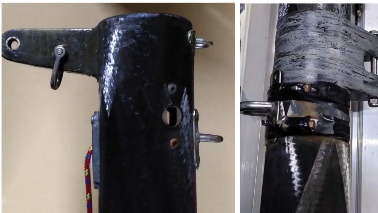
On a carbon mast, fittings can be built in, like the mast crane left, bonded on – gooseneck or clamped on – spinnaker ring.
