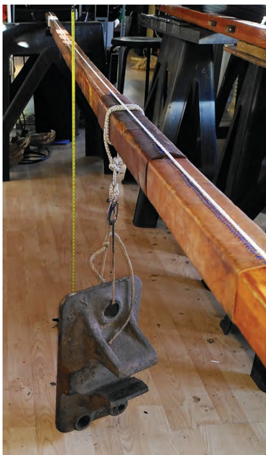
Figure 4: Measuring deflection of the existing wooden boom the old-fashioned way.
