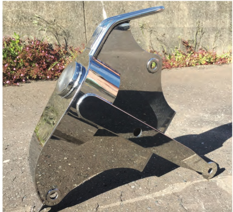
Top-down solutions – left and above: Modern masthead fitting incorporating a sheave box, crane, mounting for the navigation light and well separated attachment points for the standing rigging.
