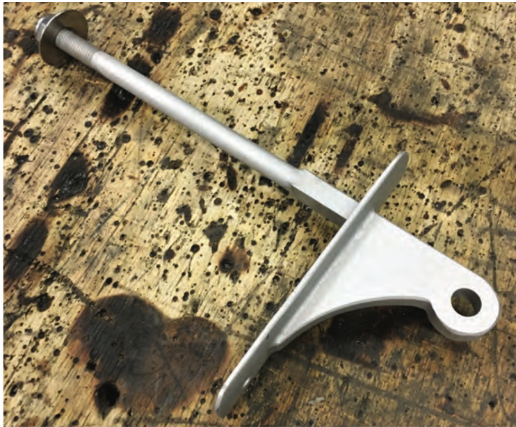
Above: A simple and stylish mast crane for the throat halyard. Note the squared section of the through-bolt to prevent the crane from twisting under load.
