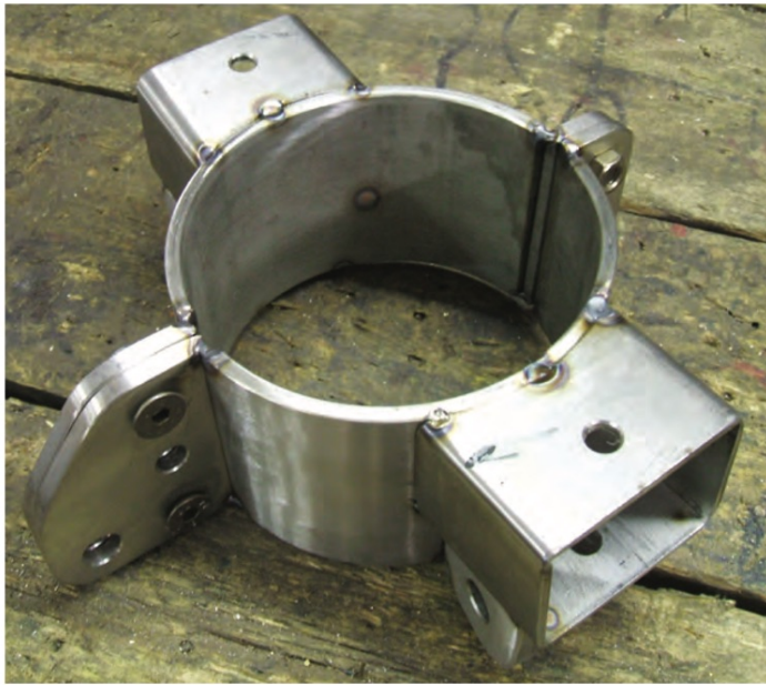
Above: Again this hounds fitting is split fore and aft. The spreader boxes are integral with the shroud attachments. Note the drainage holes in the bottom of the boxes. Halyard and backstay lugs still to fit. This example was shouldered on. Below left: Bermudan rigs can't use bolting flanges, so this fitting is through bolted at the top for diamond stay lugs, below for lower shrouds. Below right: A busy time in the workshop, with stainless mast furniture and a bronze gooseneck band.
