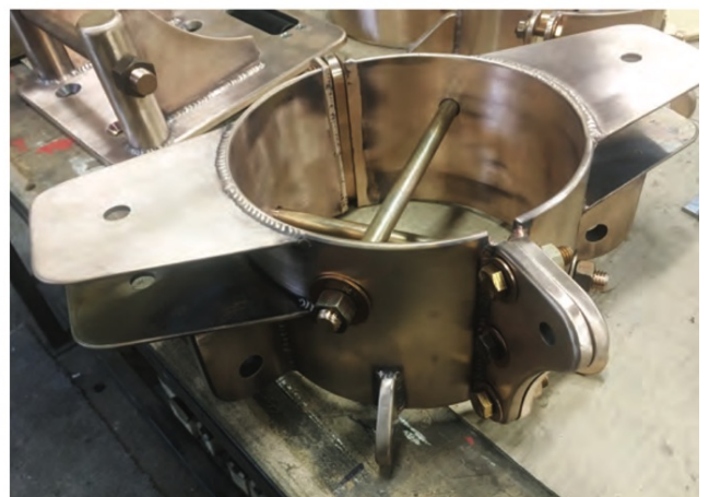
Below: Here attachments for the spreaders are incorporated into a hounds fitting. Note the fore and aft bolted flanges with the forward flange increased in size to include a crane for the head stay. This one is fixed with through bolts and friction.
