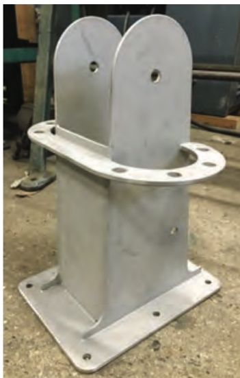
Above left: A typical deck-stepped arrangement with cleats on the tabernacle. Above right: Or leading the lines aft from the base of the tabernacle to the cockpit, this time on Andrew Wolstenholme's own boat, Kite. Left: Or then again incorporate a pinrail instead of cleats.
