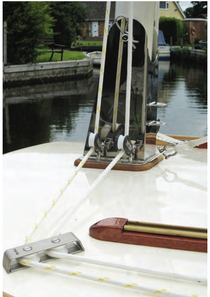
Above left: A typical deck-stepped arrangement with cleats on the tabernacle. Above right: Or leading the lines aft from the base of the tabernacle to the cockpit, this time on Andrew Wolstenholme's own boat, Kite. Left: Or then again incorporate a pinrail instead of cleats.
