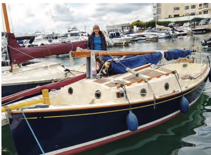
Above: On the Yare & Bure One Design – or 'White Boat' – the tabernacle sides extend down to the keel and the pivot is set low enough to allow the foot of the mast to swing up under the foredeck. Photograph: Andrew Wolstenholme. Below: The mast lowered on the Norfolk Gypsy. Courtesy: Neil Thompson Boats.
