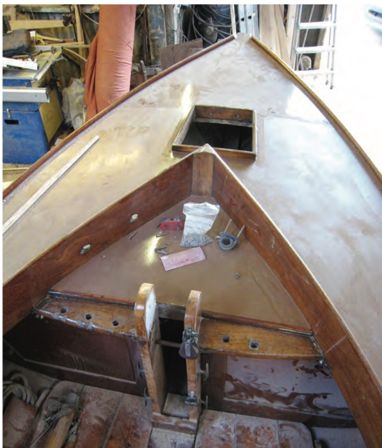
Above: On the Yare & Bure One Design – or 'White Boat' – the tabernacle sides extend down to the keel and the pivot is set low enough to allow the foot of the mast to swing up under the foredeck. Photograph: Andrew Wolstenholme. Below: The mast lowered on the Norfolk Gypsy. Courtesy: Neil Thompson Boats.
