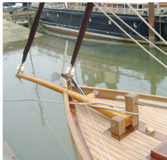
Above left: This traditional arrangement has the bowsprit heel sandwiched between bitts which extend down to the keelson. Right: Here brought up to date. Below: Modern fitting for a fixed heel. Bottom: Roller fitting for a retractable bowsprit.
