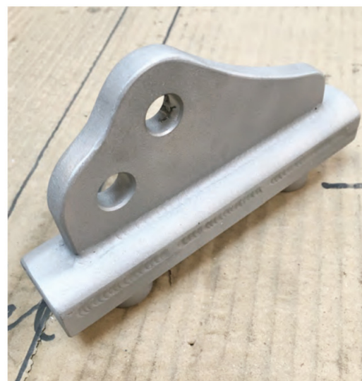
Above: Cranse iron for a Dublin Bay 25. Below: Bobstay fitting to go with it.
