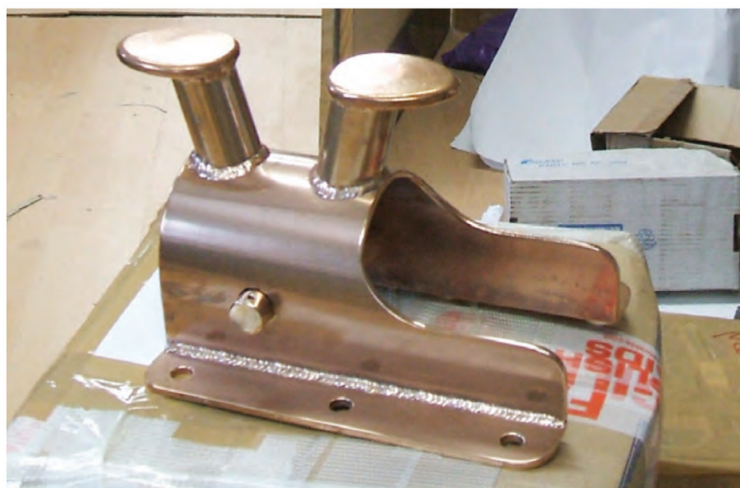
Above left: This traditional arrangement has the bowsprit heel sandwiched between bitts which extend down to the keelson. Right: Here brought up to date. Below: Modern fitting for a fixed heel. Bottom: Roller fitting for a retractable bowsprit.
