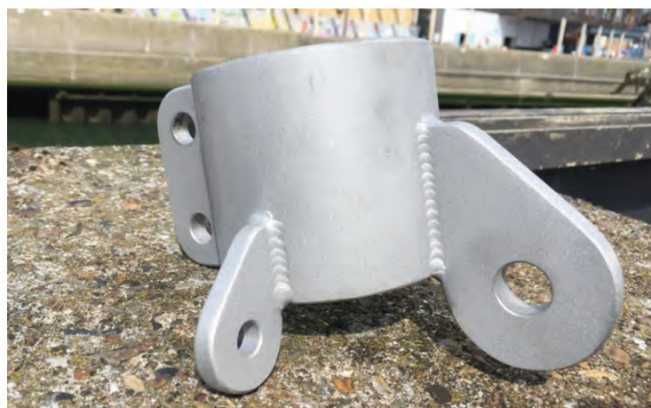
Above: Cranse iron for a Dublin Bay 25. Below: Bobstay fitting to go with it.
