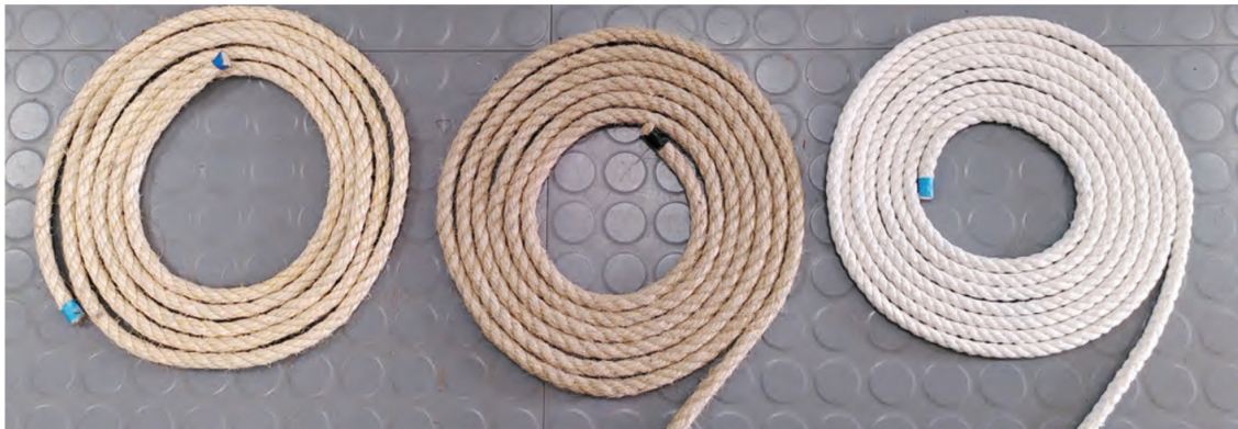
Old favourites! Above: left to right, sisal, hemp and cotton. Below: Coir is the natural fibre rope most widely used for fenders.
