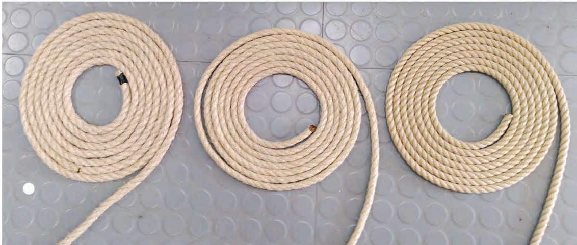
Above: New favourites: from left to right, hemp, polypropylene and polyester. Below: 'Normal' nowadays: braided polyester in a variety of colours and finishes
