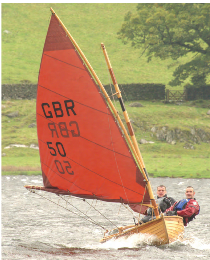
Above left: The International 12 uses a boomed standing lug, here being driven quite hard – Good Wood Boat Co. Above right: If the yard of a standing lug is attached to the mast by jaws it's a gunter rig, like this Mirror dinghy used as a trainer at Restranguet SC – Martin Egan. Below: Lymington River Scows have developed their lug rig over decades to provide very close racing – photo Coolhat Photography. Facing left: Nigel Irens was one of the first designers to update the lug rig for larger craft. Here is his elegant and fast 30' (9m) Roxane – Kathy Mansfield. Facing right: Michael Storer was inspired by the late 19th century American canoeists to design his Beth canoe – Jon Armstrong.
