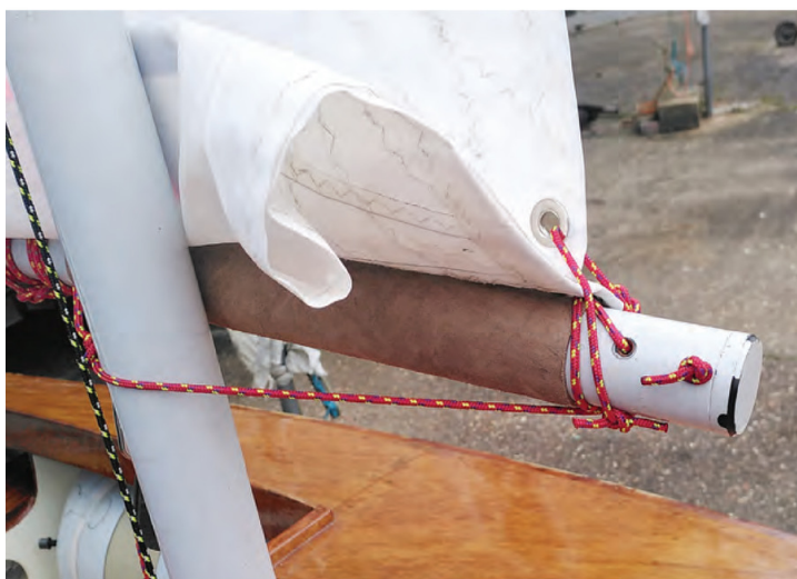
Above left Figure 4: It is simple enough to drop a loop over the front end of the boom. Figures 5a – above right – and b & c below: The after reef pendant led through the leech cringle around the boom and back through the same side of the sail. Then aft to the cleat. When tensioned the bunt of the sail falls clear.
