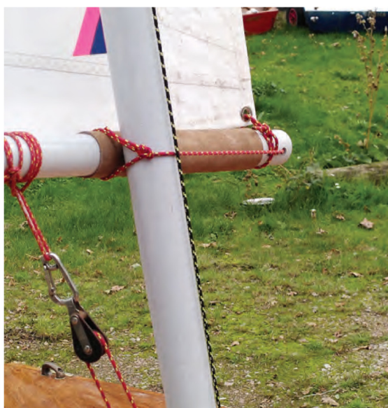
Above left: Figure 1 – A 'bleater' rigged to prevent the boom going forward also allows the boom height to be adjusted freely. Right: Figure 2 – The downhaul – still a work-in-progress – fitted aft of the mast to reduce sail twist. Below: Figures 3a & 3b – The 1880s canoeists did like to complicate things but their roller furling battened mizzen anticipated the gear fitted to modern yachts.
