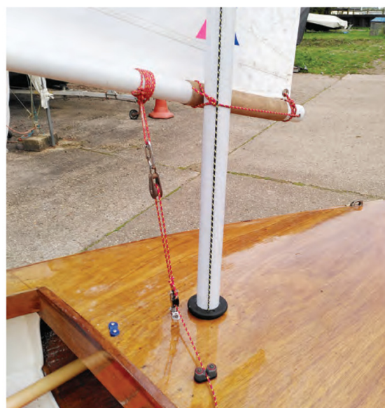
Above left: Figure 1 – A 'bleater' rigged to prevent the boom going forward also allows the boom height to be adjusted freely. Right: Figure 2 – The downhaul – still a work-in-progress – fitted aft of the mast to reduce sail twist. Below: Figures 3a & 3b – The 1880s canoeists did like to complicate things but their roller furling battened mizzen anticipated the gear fitted to modern yachts.
