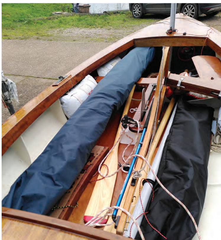
Above Figure 6: The reef tucks in neatly and quickly. Below Figure 7: Nearly all the rig packs away neatly: blue bag for mainsail, yard and boom; black one mizzen sail, spars and boomkin. The mainmast becomes the ridge pole for the boat cover.
