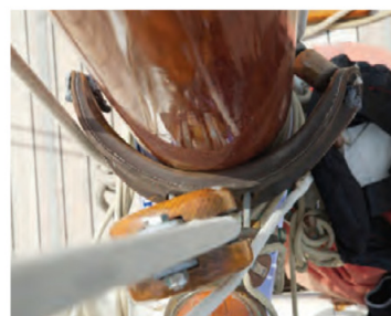
Figure 2: Size Matters A – A reasonably tight fitting saddle will keep loads central. B – If a little larger, loads can be applied off-centre, sometimes splaying the saddle C – Making the situation progressively worse. Below: Two real life examples!
