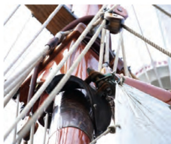
Figure 2: Size Matters A – A reasonably tight fitting saddle will keep loads central. B – If a little larger, loads can be applied off-centre, sometimes splaying the saddle C – Making the situation progressively worse. Below: Two real life examples!
