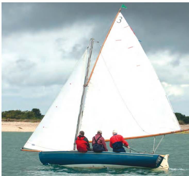
Above – Figure 3: Note the topping lift loop running to the masthead – slack when the sail is set. See also the tell tales setting well at the head of the sail.
