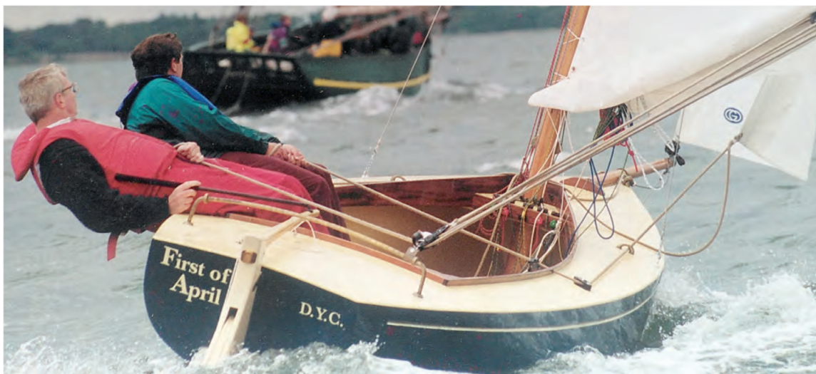
Above: The author's Orwell Corinthian. A larger mainsail needs more purchase: here a 4:1 system on a horse. Photo: Kathy Mansfield. Below: Loose-footed boomless sails, like these on the St Ives Lugger Barnabas, need to be sheeted well aft. Photo: Cat Holman.
