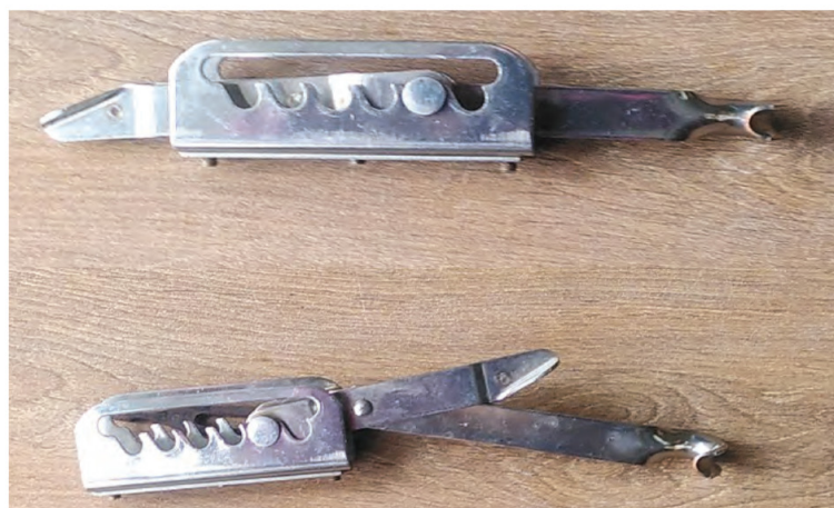
The Highfield Tensioner, much used in dinghies is an over-centre device, shown here tight (above) and loose (below). It works well on a wire halyard incorporating an eye.
