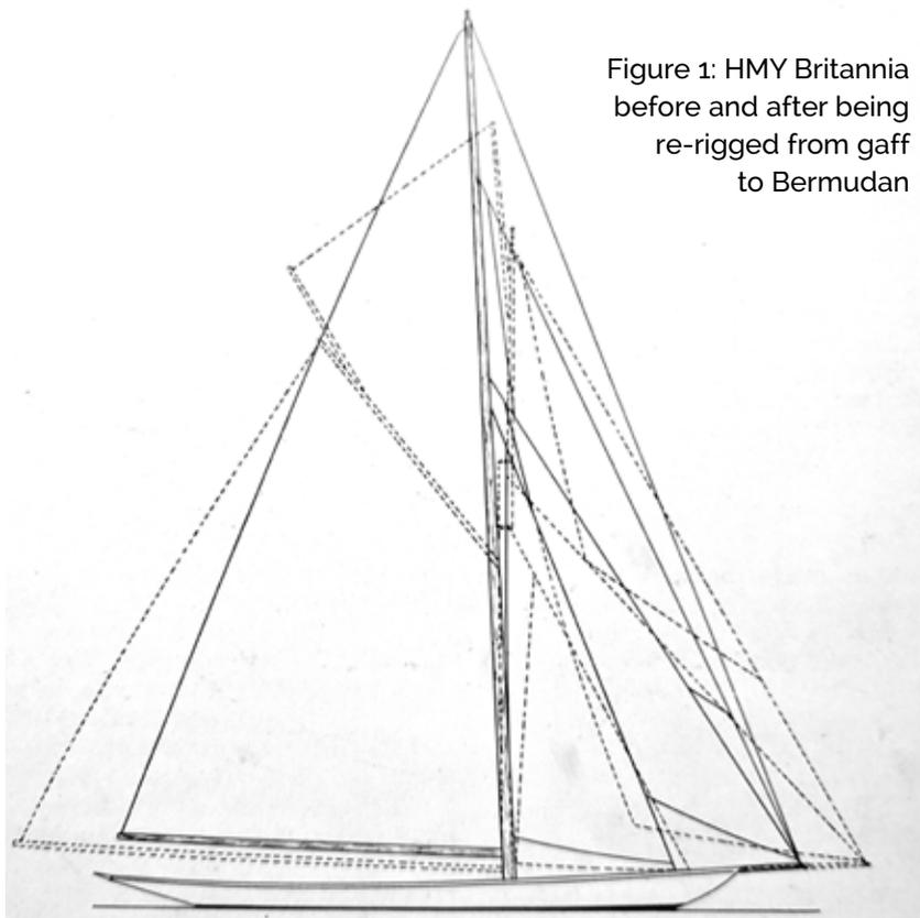
Figure 1: HMY Britannia before and after being re-rigged from gaff to Bermudan
