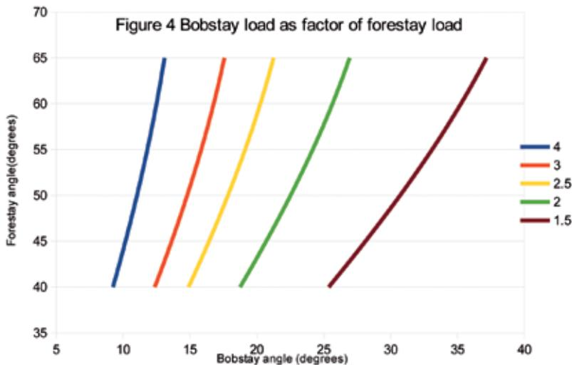
That gives us just over 13 tonnes compression in the bowsprit. Note that even on an 8 tonne boat with a moderate bowsprit, we have bowsprit and bobstay loads a good deal greater than the displacement of the boat.
